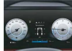
Tyre pressure monitoring system: Highline
