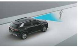
Forward Collision - Avoidance Assist - Pedestrian (FCA-Ped) Forward Collision - Avoidance Assist - Cycle (FCA-Cyl)
